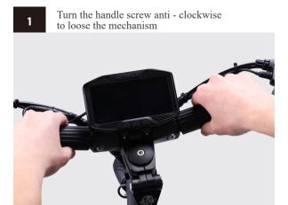
Simultaneously fold the handle bar down
