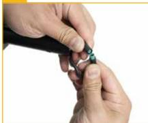
Install the accelerator clip (pay attention to the notch direction of the clip)
