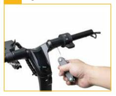
Tighten the handlebar on the right
