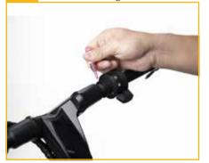
10 Tighten the headless screw below
